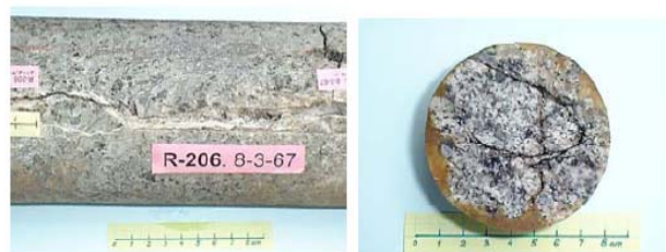
Figure 8: Natural fractures in basement rock from White Tiger field (from Chan et al., 2006).
