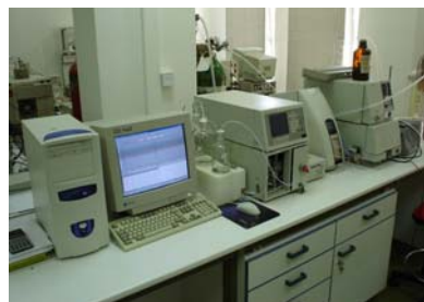
Waters high pressure liquid chromatograph (HPLC) with RI, IR, UV-DAD and ELS detectors
