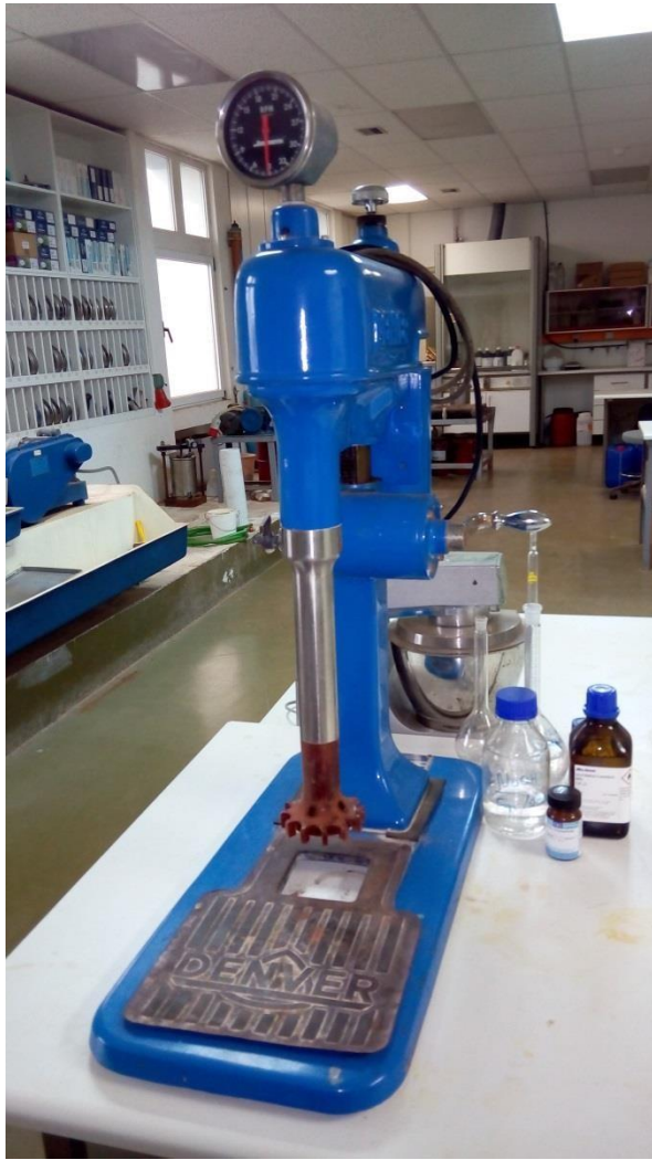
Laboratory flotation machines (Denver)
